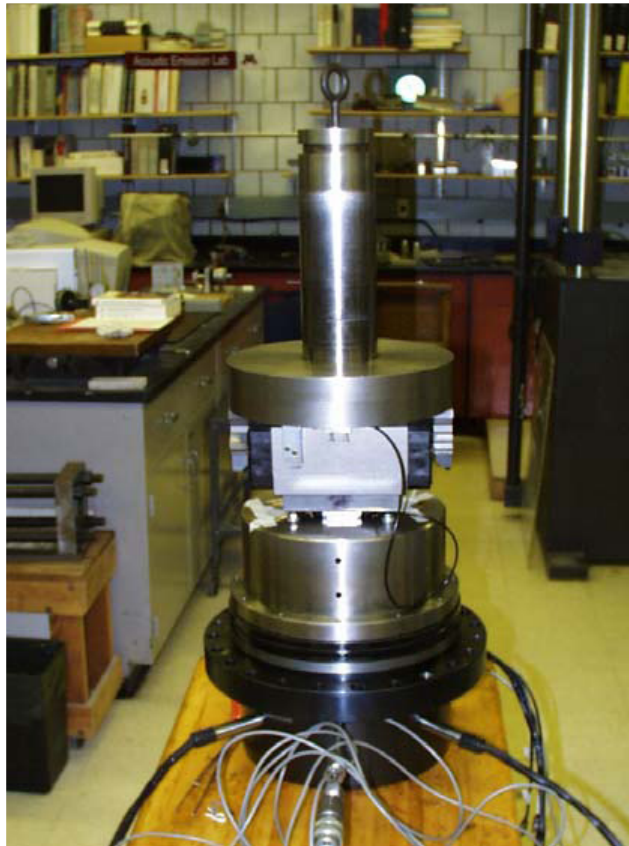
Figure 1. A novel apparatus will be used to produce faulting of fluid-saturated rock to devise rock characterization techniques and develop predictive models for the simulation of fluid-driven fractures.
