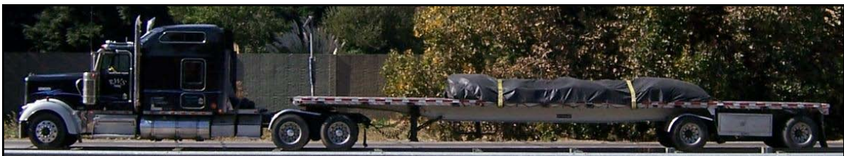
Figure 12. Photo. Class 9, Type 3S2 with “spread” rear tandem.
