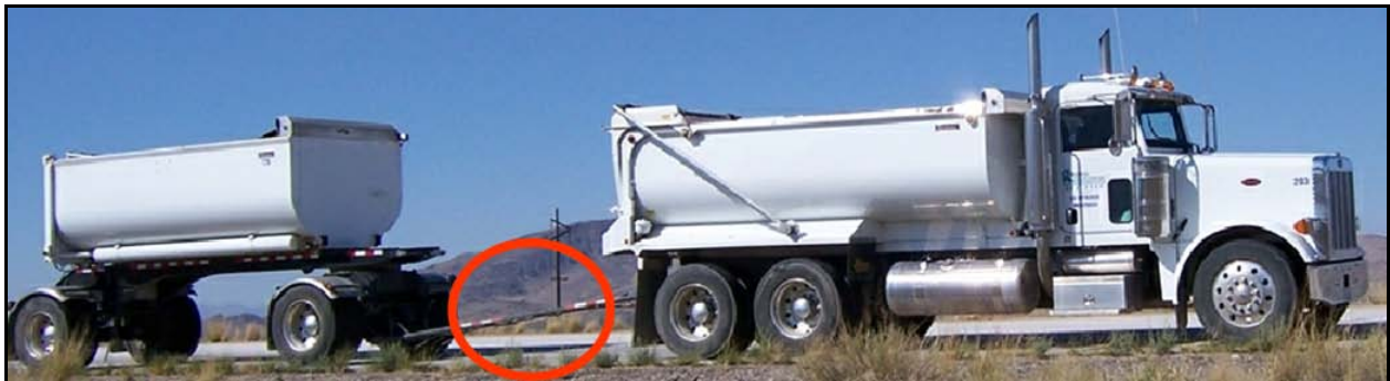
Figure 38. Photo. Class 9 Type 32 with long towbar.
