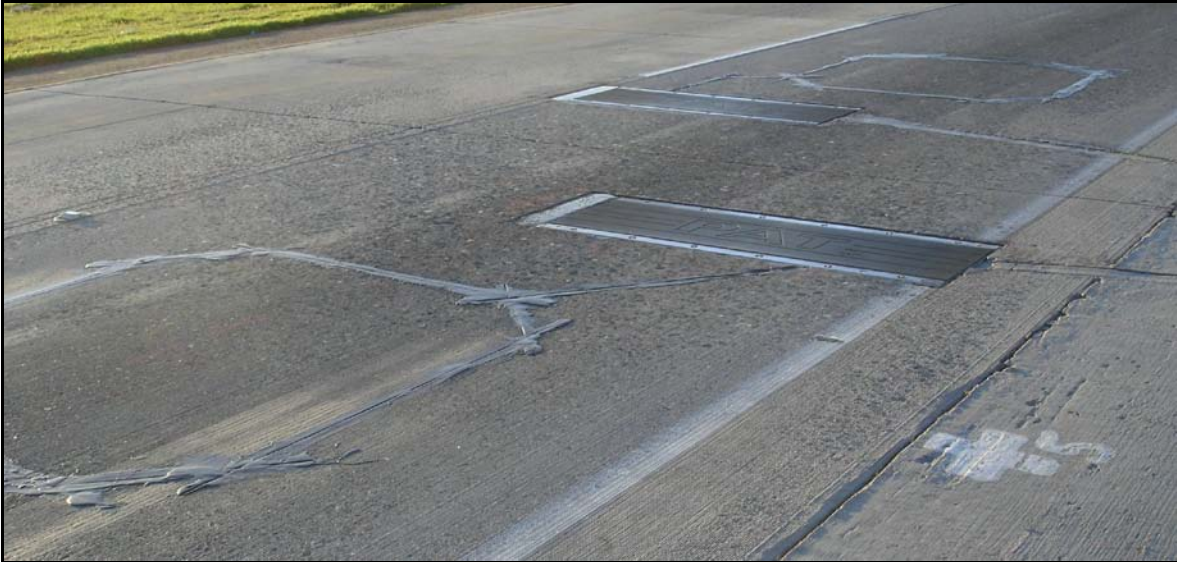
Figure 2. Photo. Staggered weigh sensors (bending plates) and detection loops (single threshold system).
