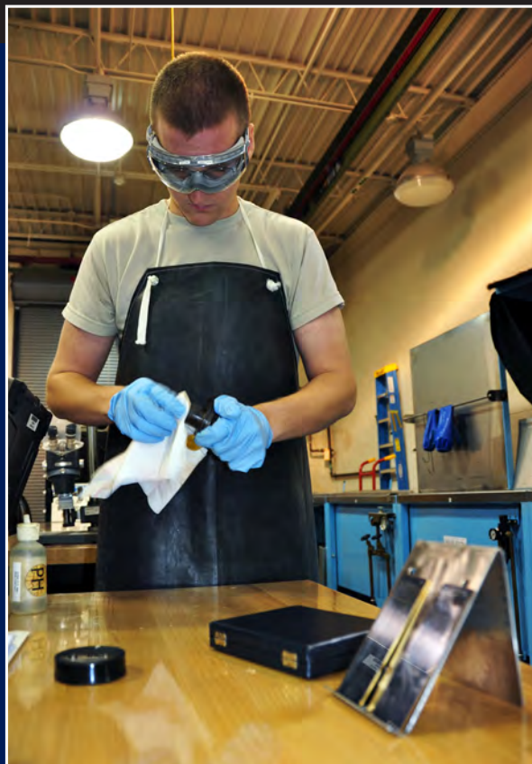
(Above) Staff Sgt. Kim Leslie, 94th Airlift Wing non-destructive inspection specialist, calibrates an eddy current machine, which will be used to detect cracks in metal parts of airframes. NDI specialists use eddy current machines, magnetic particle machines, ultrasonic detectors and portable X-Ray devices to peer into the aircraft and components without having to take them apart.
