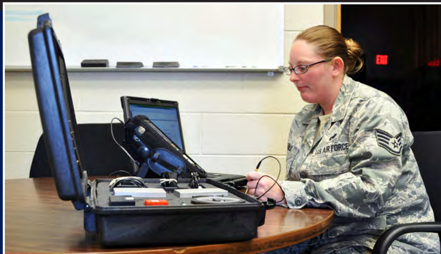
(Above) Staff Sgt. Kim Leslie, 94th Airlift Wing non-destructive inspection specialist, calibrates an eddy current machine, which will be used to detect cracks in metal parts of airframes. NDI specialists use eddy current machines, magnetic particle machines, ultrasonic detectors and portable X-Ray devices to peer into the aircraft and components without having to take them apart.
