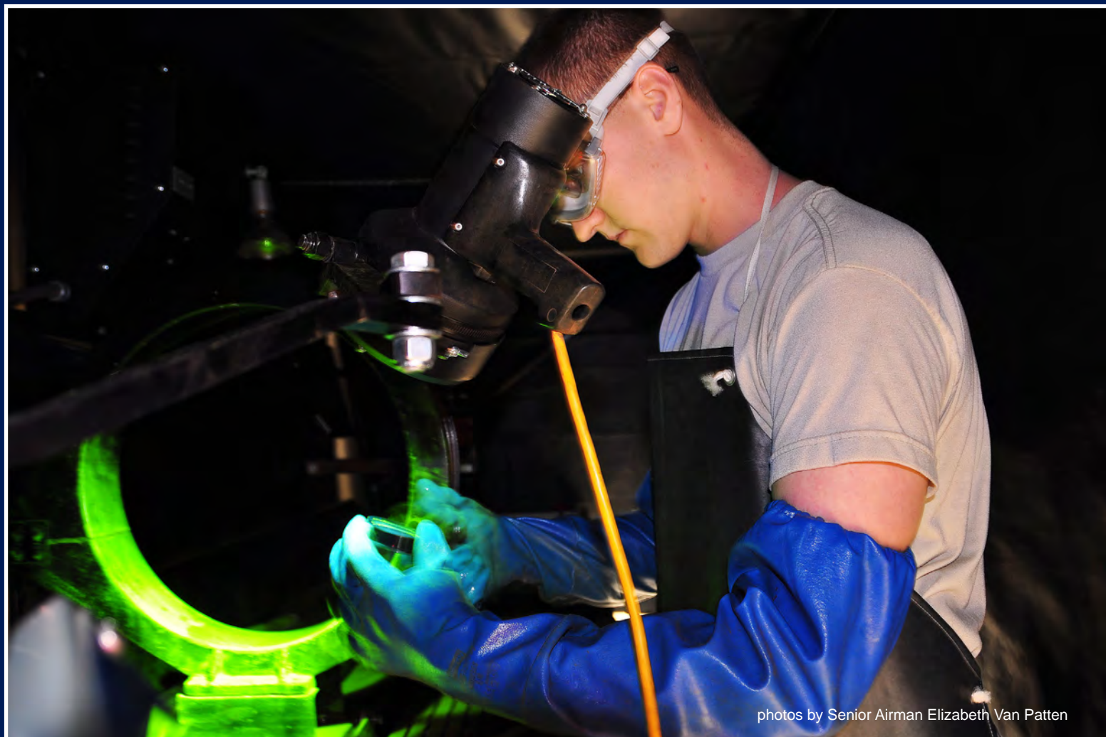
(Below) Airman 1st Class Dylan Brown, 94th Airlift Wing non-destructive inspection specialist, uses a magnetic particle machine to detect cracks on a metal test piece. Cracks on the test piece appear bright green under black light, due to liquid dye penetrant.
