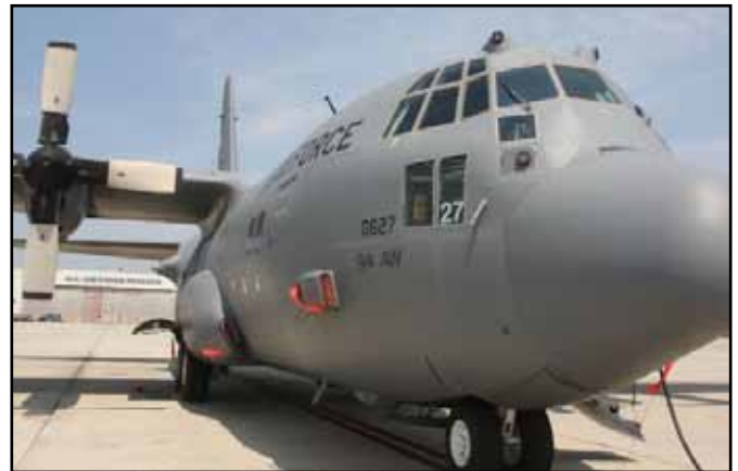
Pictured is a C-130 that has been modified. Dobbins has installed the Large Aircraft Infrared Counter Measures system which protects vulnerable, large and slow-flying aircraft from missile attack. (U.S. Air Force photo/ Don Peek)
