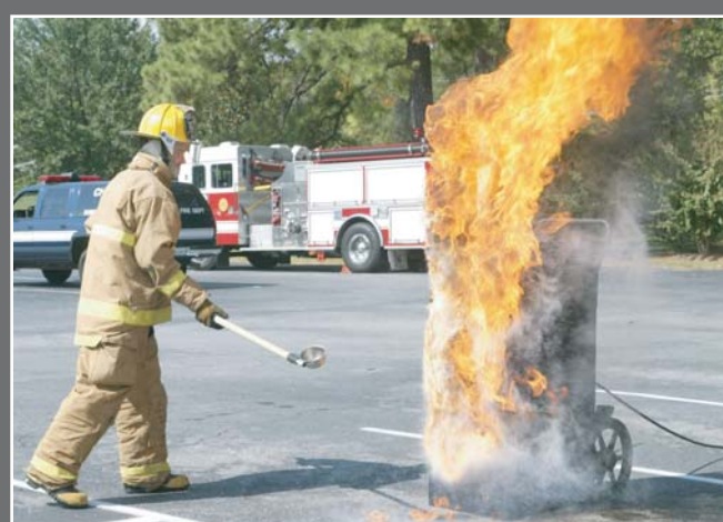
A firefighter from the Dobbins Fire Department demonstrates the results of applying water to a grease fire using a simulator developed by one of Dobbins' own.
