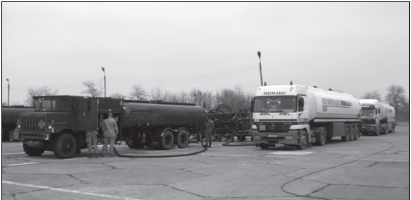
A commercial tank truck downloads fuel to a U.S. Air Force mobile refueler at Bezmer Air Base, Bulgaria.
