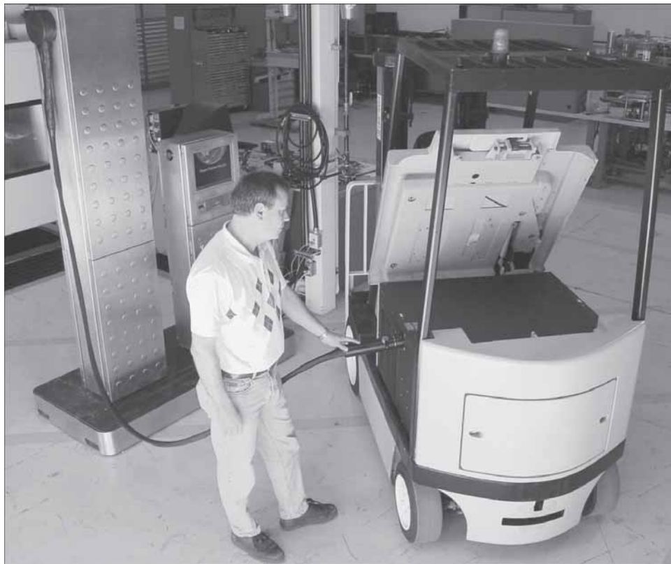
A Defense Distribution Center Susquehanna warehouse employee refuels a hydrogen cell technology forklift at the facility in New Cumberland, Pa. (Courtesy photo)
