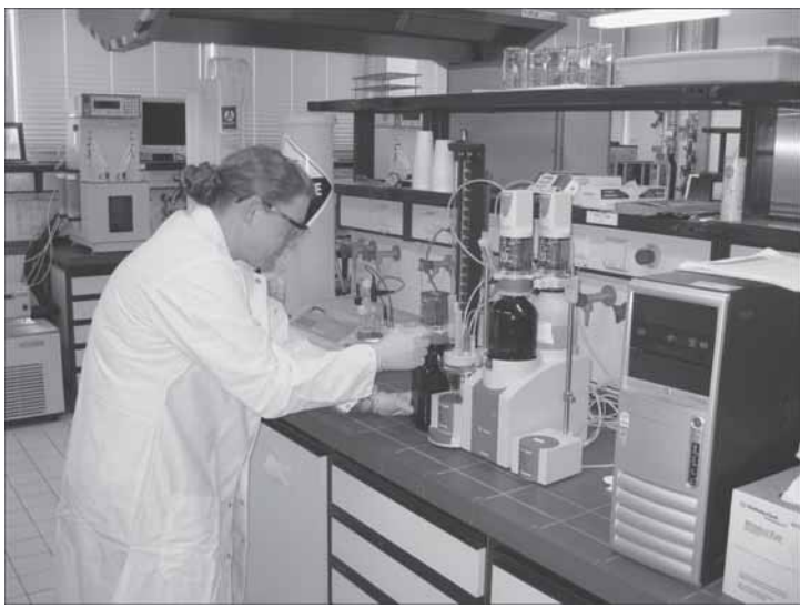
Army Staff Sgt. Barbara Mooney performs total acid number testing of a JP8 fuel sample in the Defense Energy Support Center Europe Petroleum Laboratory, Kaiserslautern, Germany.
