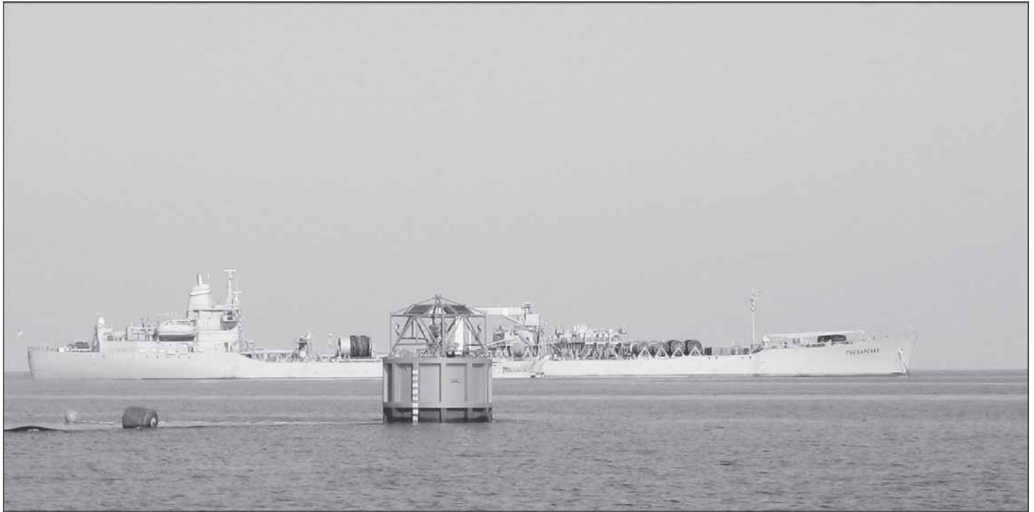
The Single Point Mooring System buoy after being launched by the SS Chesapeake, which passes behind the buoy. (Courtesy photo)
