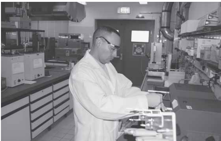
Army Cpl. Sergio Gonzalez, A Company 1-185 AR, performs density analysis of a jet fuel sample.
