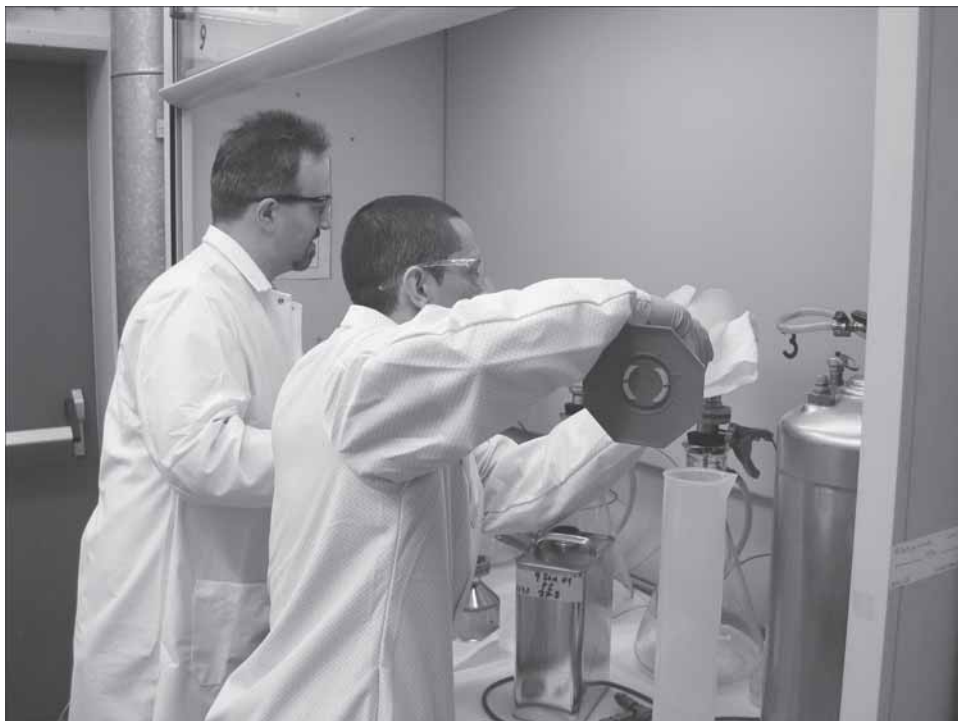
Axel Spear and Specialist Gilbert Lopez of the Defense Energy Support Center Europe Petroleum Laboratory perform particulate contamination and filtration time testing of a JP8 fuel sample. (Courtesy photo)
