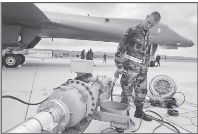
Airman 1st Class Charles Gann, a Ramstein Air Base, Germany, fuels specialist, uses a pantograph to refuel a B-1 Lancer. Defense Fuel Support Points, like the one on Ramstein, enable local and transitory customers to pay for the fuel only when they use it. (U.S. Air Force photo by A1C Marc I. Lane)
