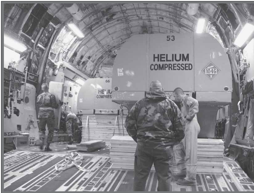
Robert Gloria, a transportation management specialist in the Defense Energy Support Center's Aerospace Energy Commodity Business Unit, watches as shoring kits are used to secure a bulk helium trailer aboard a U.S. Air Force C-17 at Lackland Air Force Base, Texas. (Courtesy photo)
