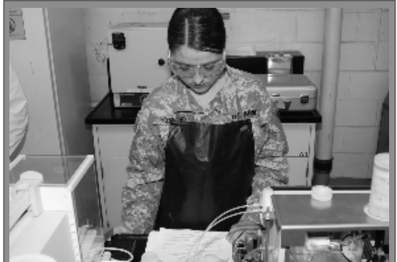
Army Pvt. Masha Hosford, a petroleum laboratory specialist student, performs a fuel density test in one of the labs at the Fort Lee, Va., Petroleum and Water Department school.
