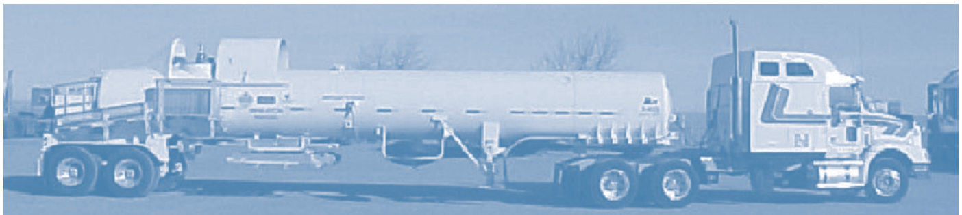
The DESC-M trailers are the only N_2O_4 and hydrazine trailers that are special permitted by DOT for over-the-road shipment.
