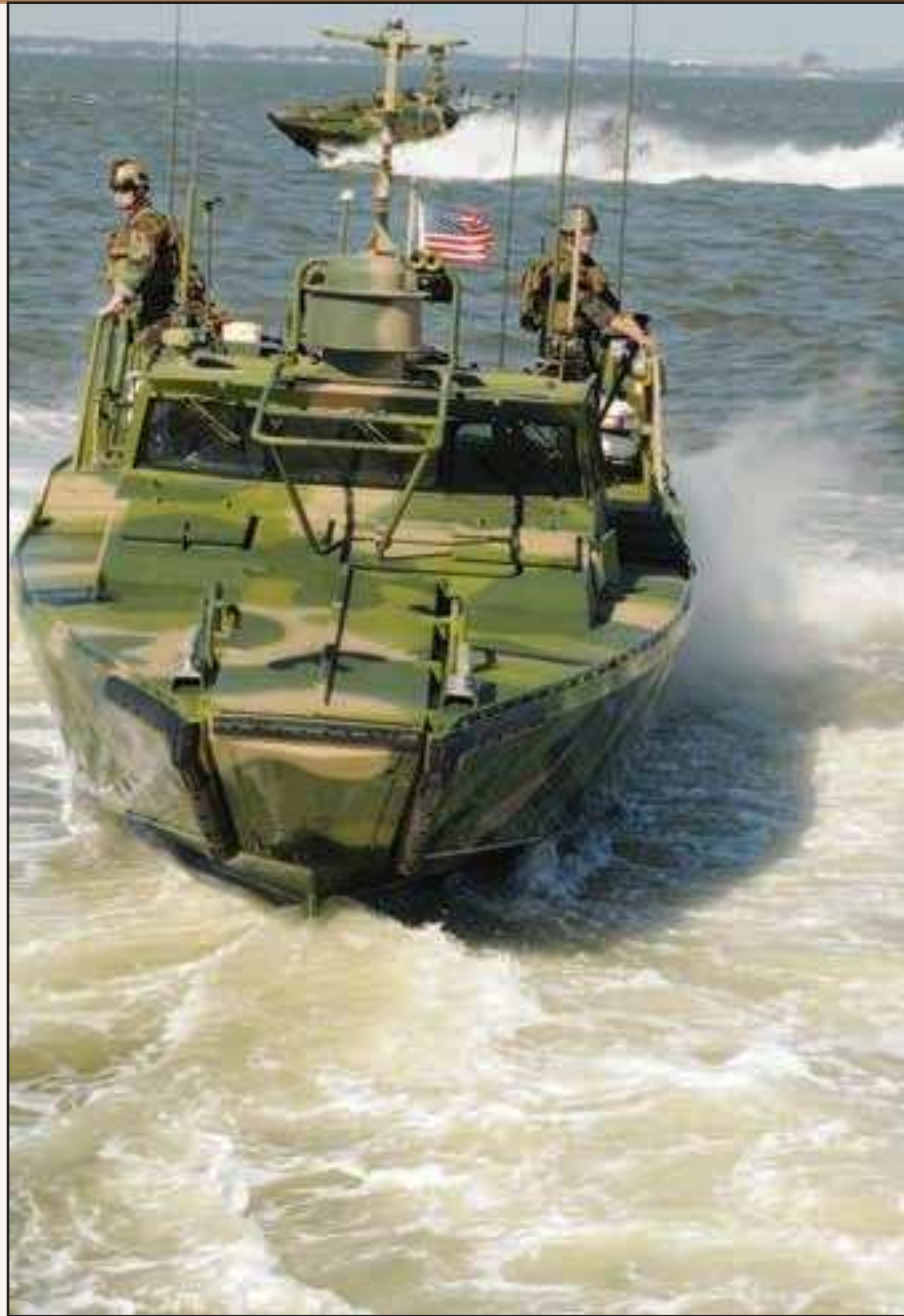
Above and left, sailors assigned to Riverine Group 1 conduct maneuvers aboard Riverine Command Boat (Experimental) at Naval Station Norfolk in Va. The craft is powered by an alternative fuel blend of 50 percent algae-based and 50 percent NATO F76 fuels procured by the Defense Logistics Agency Energy in support of the secretary of the Navy’s efforts to reduce total energy consumption on naval ships. Photo by Petty Officer 3rd Class William Jamieson.
