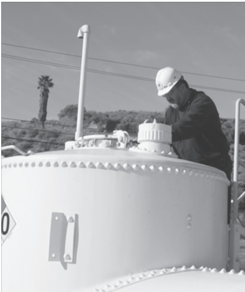
Defense Energy Support Center America's West Leo Burruel, quality assurance representative, prepares to take a fuel sample from a fuel storage tank. (Photo courtesy of DESC-AMW)
