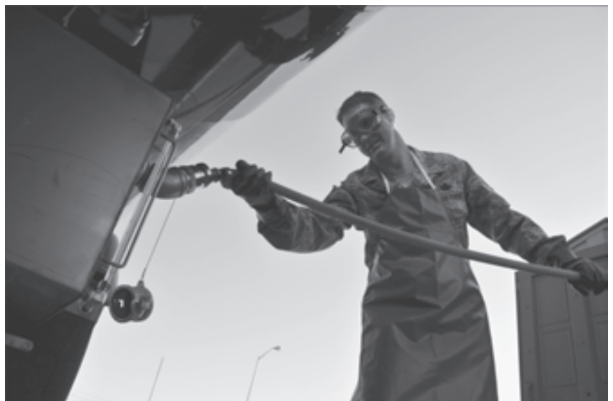
An airman at Minneapolis St. Paul Air Reserve Station, Minn., fills an additive injector tank on a refueling unit.
