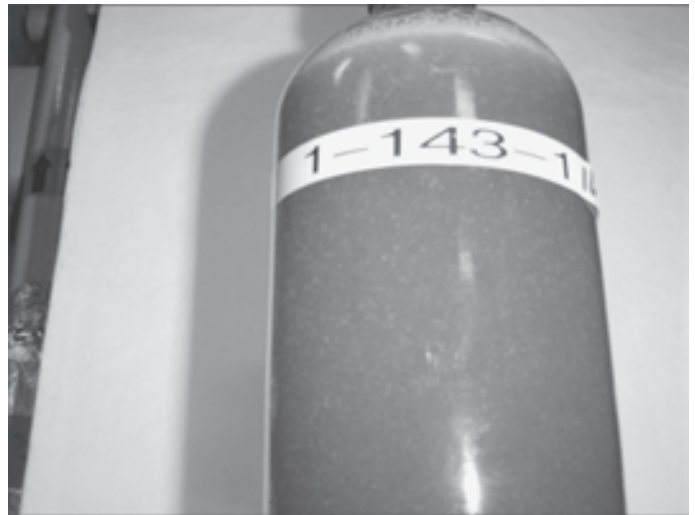
Above: This photo is an in-line sample taken from the starboard service tank, 4-143-1-F. It was taken after the fuel was exposed to two days of mid-50 degree F temperatures.
