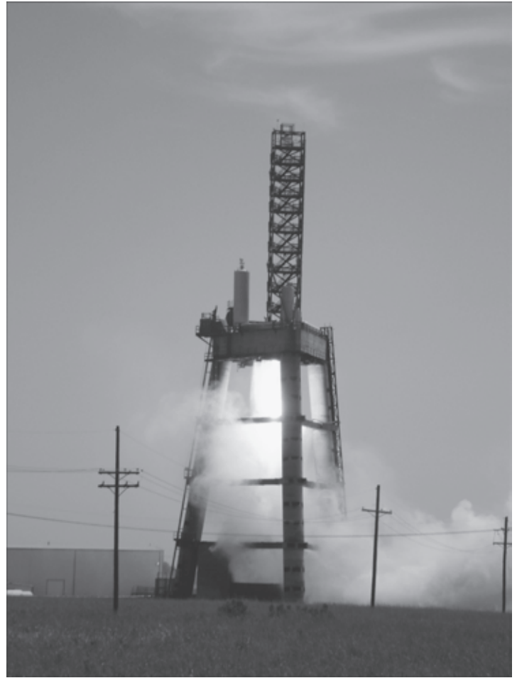
A Merlin Rocket engine test at SpaceX Corporation's McGregor, Texas, test site. (Photo by Lou Foehrkolb)
