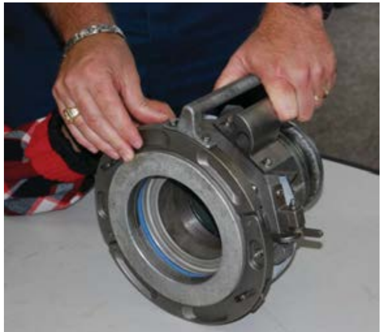
An example of the QUICKER quick disconnect coupling is examined at Yokota Air Base, Japan. Photo courtesy of DLA Energy Pacific.
