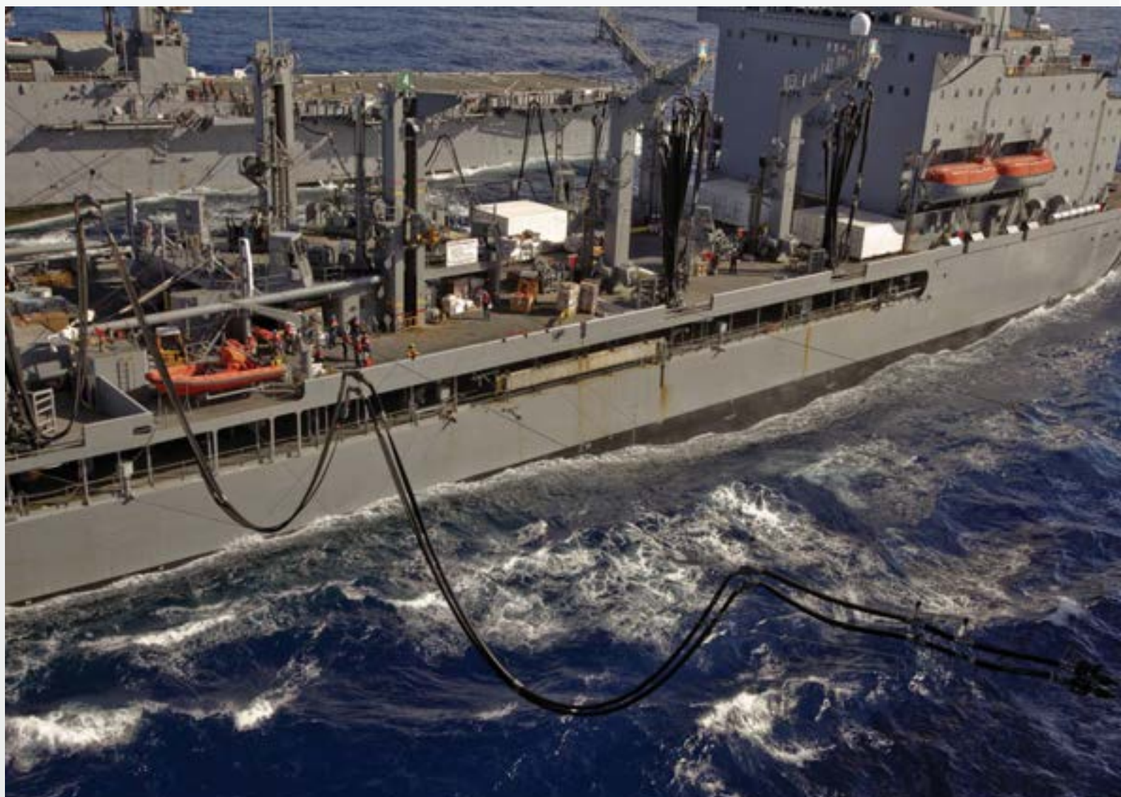
PACIFIC OCEAN (July 13, 2010) The Military Sealift Command fleet replenishment oiler USNS Guadalupe (T-AO-200) extends fuel lines toward the amphibious assault ship USS Bonhomme Richard (LHD 6) during Rim of the Pacific 2010 exercises. RIMPAC is a biennial, multinational exercise designed to strengthen regional partnerships and improve multinational interoperability. The U.S. Navy will be using 450,000 gallons of biofuel procured by the Defense Logistics Agency Energy during RIMPAC 2012 U.S. Marine Corps Lance Cpl. Orlando Perez/Released.
