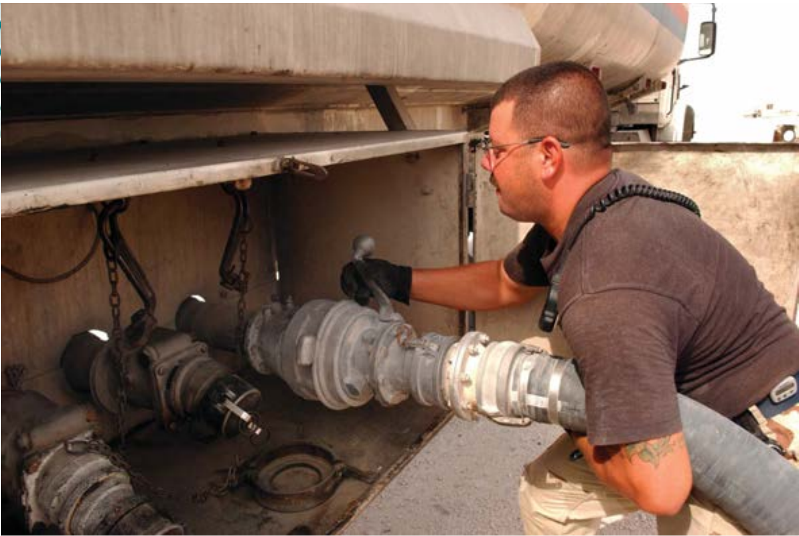
U.S. Air Force personnel with the 379th Expeditionary Logistics Readiness Squadron, hook up the 6-inch refueling hose from the R-22 fueling equipment on a commercial receipt truck, at an undisclosed location. As the largest consumer of jet fuel among the military services, the Air Force spent $7.2 billion on 2.7 billion gallons of fuel in 2010. Photo by U.S. Air Force Airman 1st Class Desiree Hayden.
