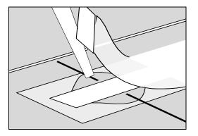
(2) Reseal the tape over the sample pad compartment. When testing multiple samples, complete the peel, pipette, and reseal steps on each strip before going to the next strip.
