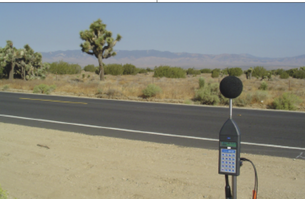
Noise measurement equipment used for “quiet pavements” research.
