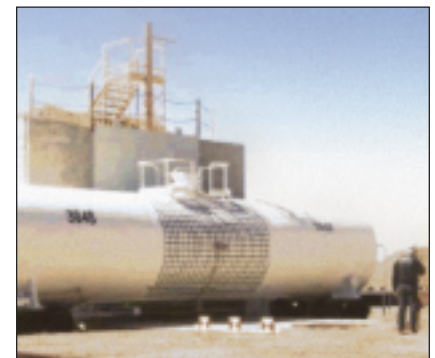
Tank car positioned for full-scale tests; the tank car contains water mixed with clay slurry to produce the density approximately equal to that of liquid chlorine.
