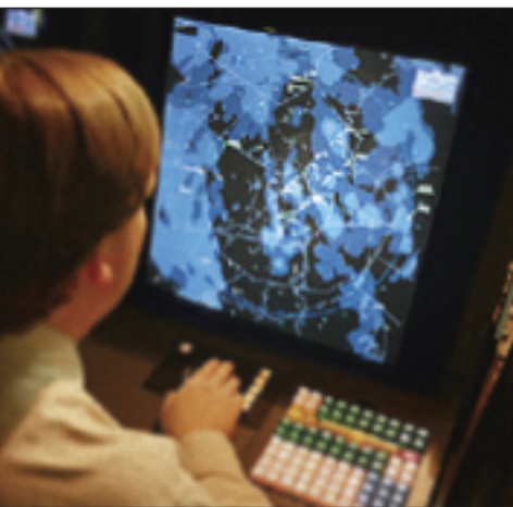
Standard Terminal Automation Replacement System (STARS). Workstation displays are configured to provide only the information needed by air traffic controllers. (photo from Raytheon Systems)
