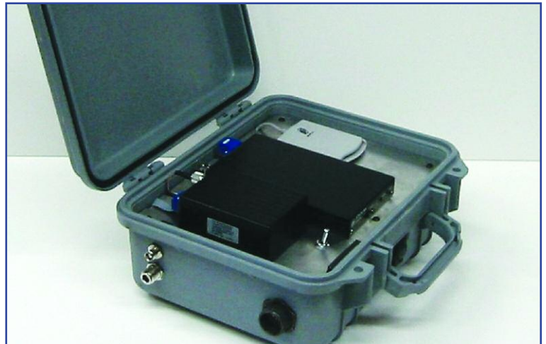
VIPS employs GPS technology in portable, highly secure transponders that are installed on authorized vessels. Each has a VHF-encrypted data link, and encryption keys are easily changed via the transponder's smart card reader. The Center designed these portable units to operate from a variety of AC and DC power sources; each also includes an internal lithium ion battery pack. Vessels equipped with VIPS are tracked on displays such as that shown below.
