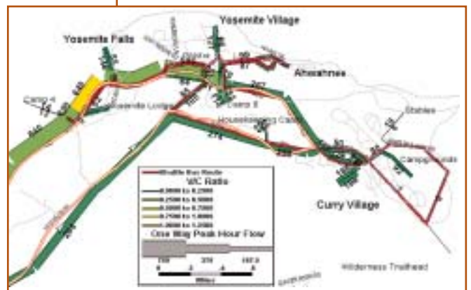
One product of Volpe's TIS project at Yosemite National Park is a network flow model. The screen shot above shows evening peak-hour traffic flow (the yellow segment depicts the congestion near Yosemite Falls), and the route of the shuttle bus.
