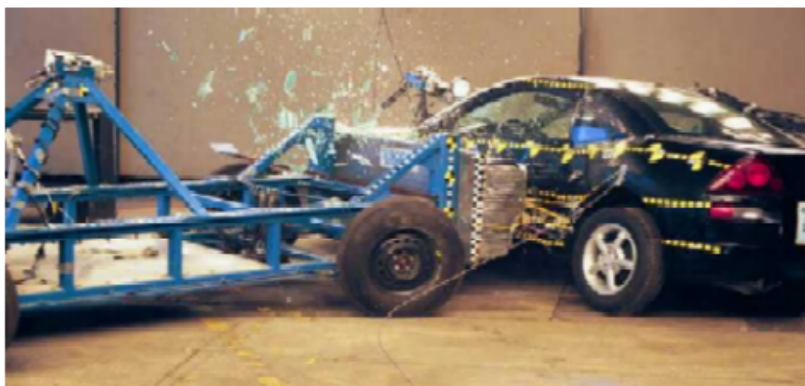
During each side-impact crash test, a moving deformable barrier designed to represent an SUV impacts a passenger car in the side at the driver's door.
