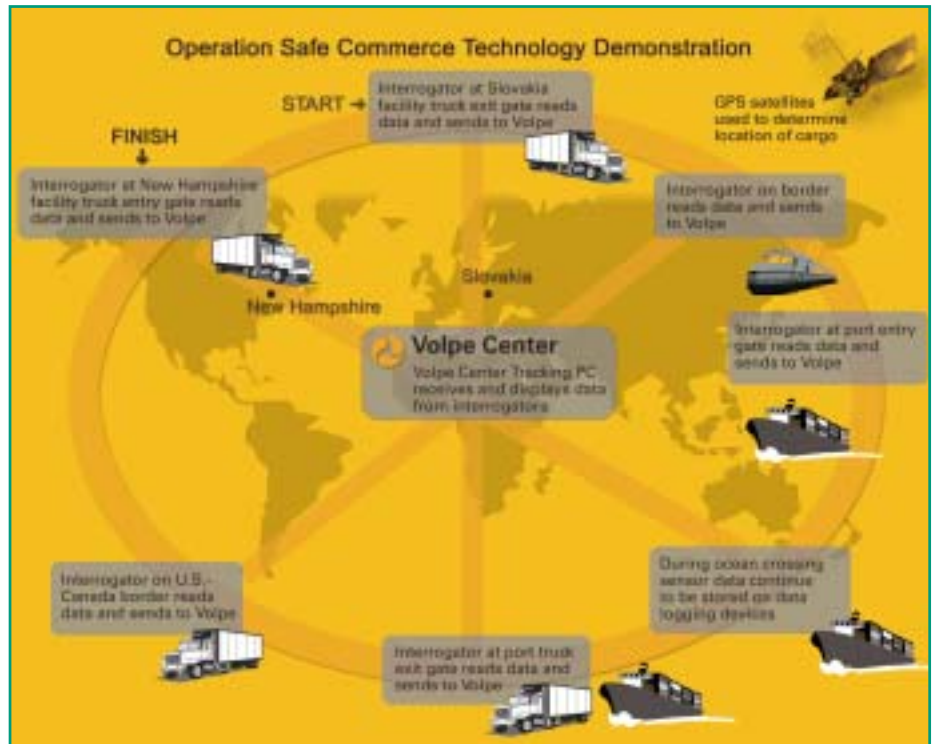
The Volpe Center manages the Entry Point Screening (EPS) Program, whose primary concern is protecting people and facilities against bombs carried by commerce, vehicles, vessels, mail, and cargo. The EPS projects include Operation Safe Commerce (above), for which Volpe performed an assessment of an entire multimodal, global supply chain and demonstrated tracking and sensing technologies. Data were captured by interrogation stations and transmitted to the Volpe Center.
