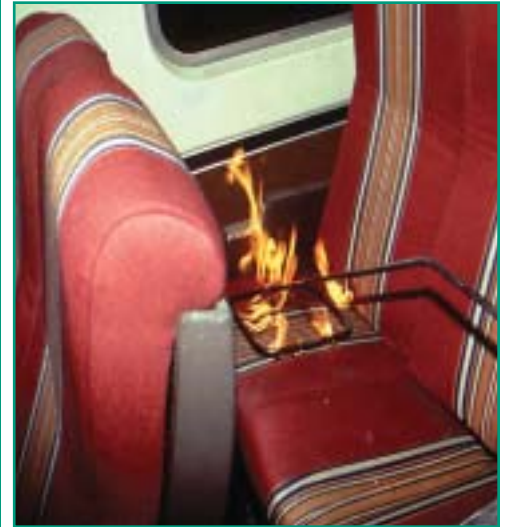
A full-scale, seat-fire test conducted on an Amtrak rail coach car, part of Volpe's support of DOT rail vehicle fire safety requirements.
