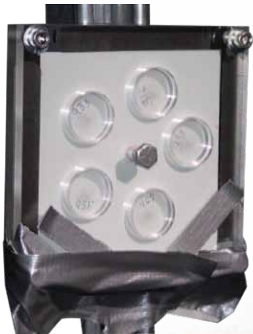
This inexpensive blast sensor developed by the Livermore team includes a plastic peak-pressure display and is designed for a single use.
