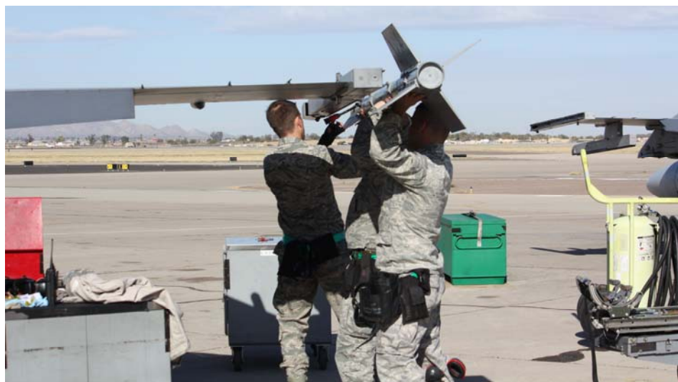
310th Aircraft Maintenance Unit Load Crew from the 756th Aircraft Maintenance Squadron loads an AIM-9 Missile.
