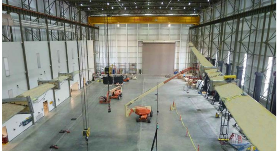
The Wind Technology Test Center in Boston, Massachusetts, is the only test center in the United States capable of testing wind turbine blades up to 90 m in length to IEC standards. Here, the test center is preparing two 49-m blades for testing. The blade on the left is being prepared for a flapwise static test and the blade on the right for an edgewise fatigue test. Photo from Nathan Post, WTTC
