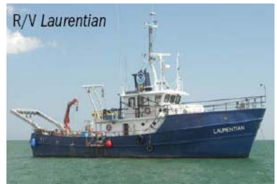
R/V Laurentian was one of the first NOAA research vessels converted to operate on bio-based fuel and lubricants.
