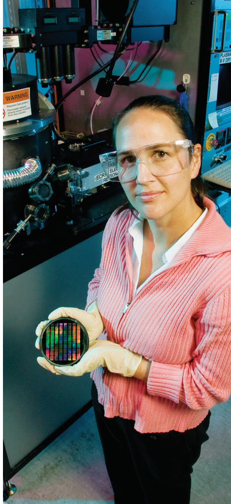
Rebecca Nikolić and her team are developing a detector made of silicon pillars and boron for capturing neutrons.
