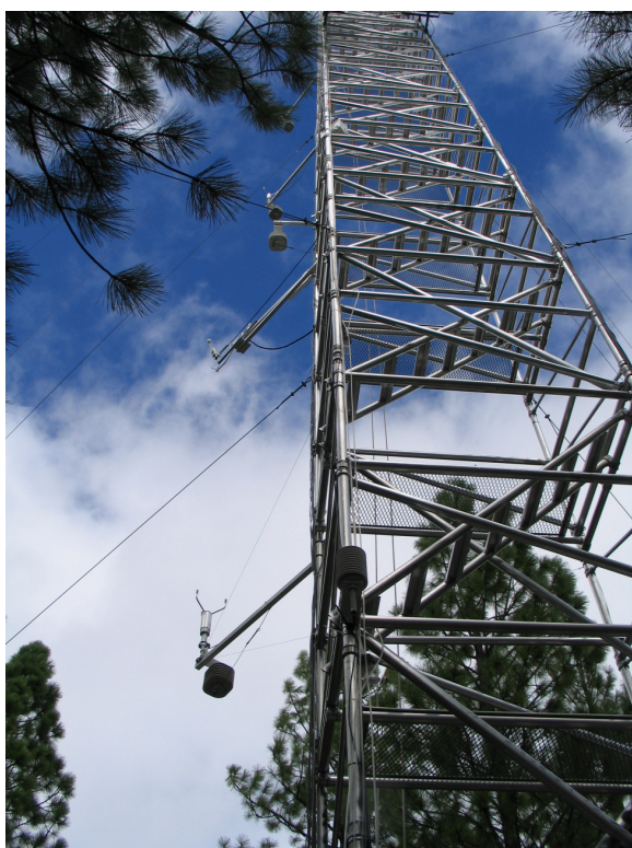
Photo 4 - AmeriFlux: the eddy covariance flux tower in Oregon ( Metolius ponderosa pine forest)- (Photo by Beverly Law).
