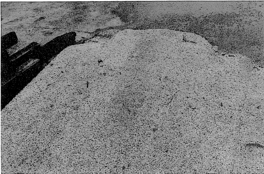
Figure 7. Close-up of skid resistance test strip of pervious concrete showing surface texture
