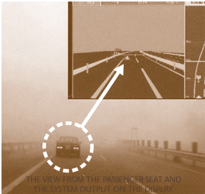
Figure 24. Driving support system—poor visibility. (Ministry of Land, Infrastructure, and Transport, Japan)
