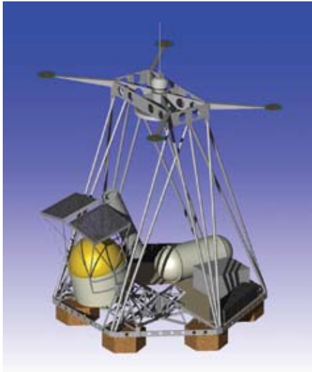
ProtoEXIST, a balloon borne instrument to develop technology for the Energetic X-ray Imaging Survey Telescope (EXIST) mission, shown in an artist's rendering. EXIST is a candidate for the Black Hole Finder Probe and will conduct a census of black holes in the known universe.
