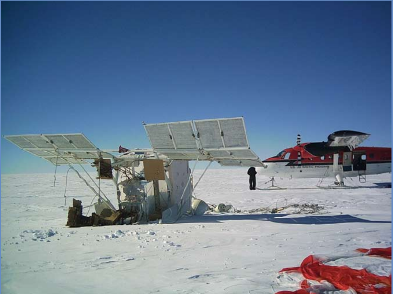
The CREAM instrument after landing in Antarctica in January 2005. Several flights of the Twin Otter aircraft are required for recovery of such instruments.
