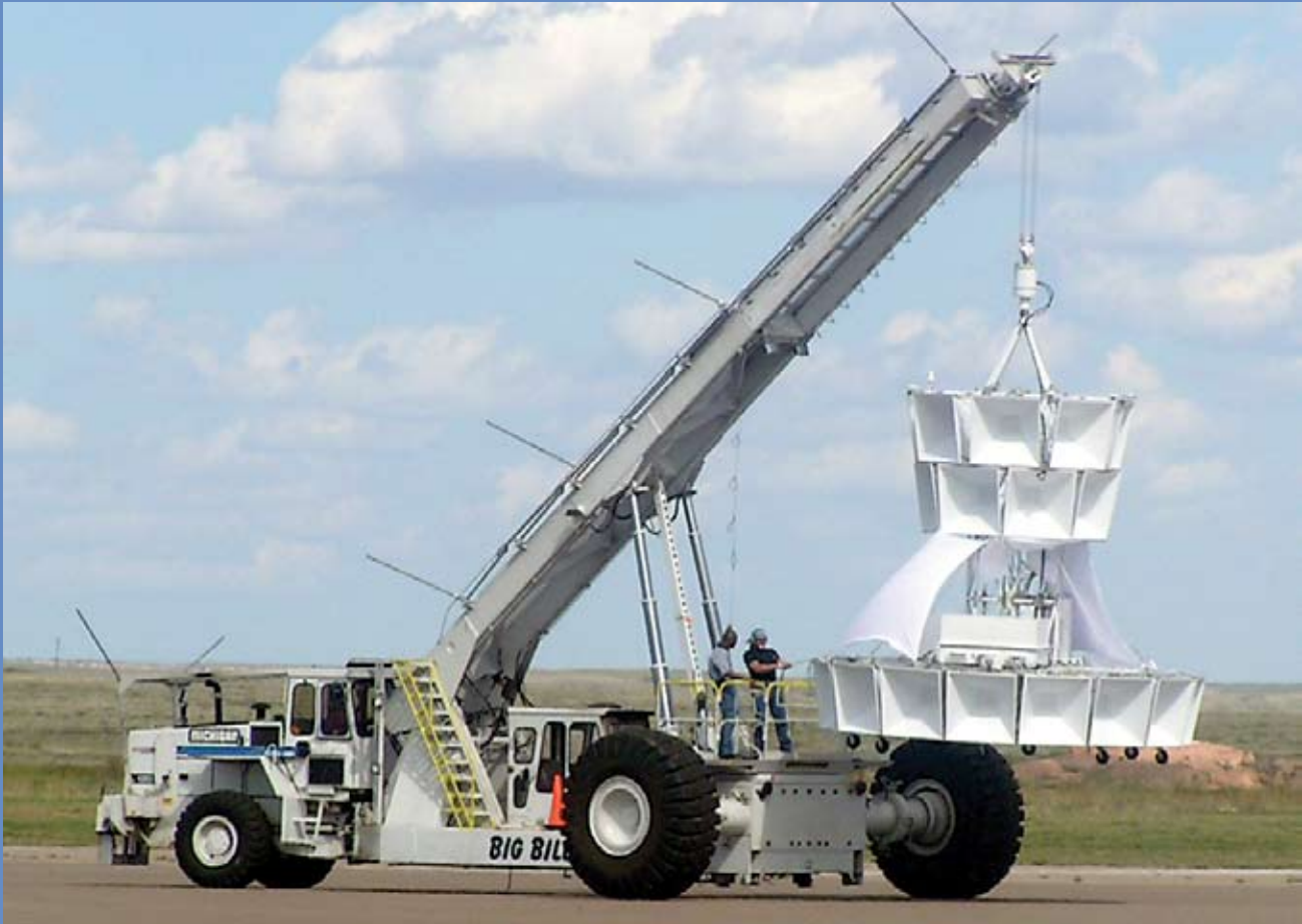
The engineering test model of the ANtarctic Impulsive Transient Antenna (ANITA) preparing for its successful August 2005 test flight. ANITA will search for pulses of radio emission from neutrinos penetrating the Antarctic ice.
