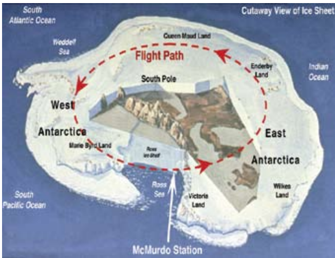
The projected path of ANITA around the Antarctic continent. ANITA looks at radio pulses from neutrinos interacting in the ice.
