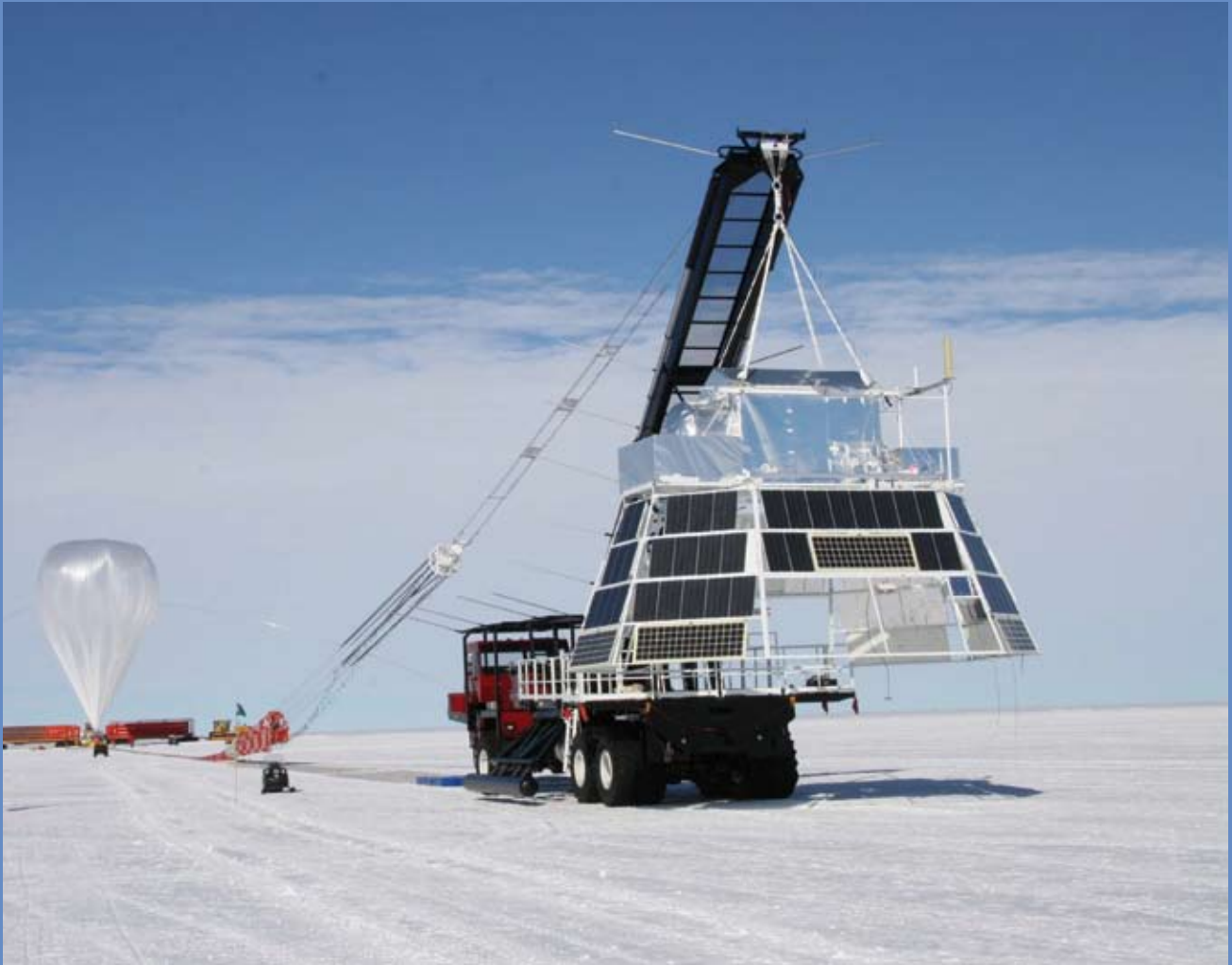
The Balloon-borne Experiment with a Superconducting Spectrometer (BESS) payload, about to launch from Antarctica. BESS has been measuring the antimatter (antiprotons) component of the cosmic rays and looking for signatures of dark matter.
