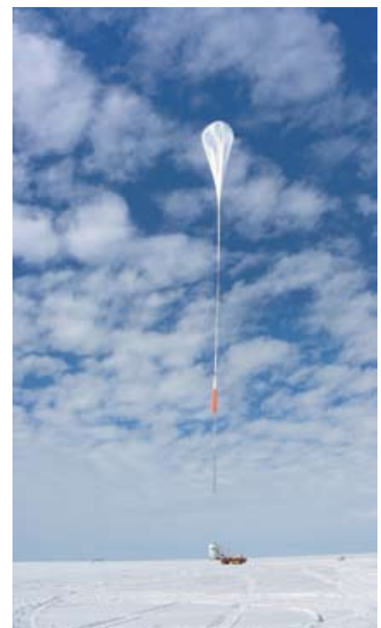
A balloon has just been released (left), and moments later lifts the instrument payload off the launch vehicle (right). In the right-hand photo the parachute hangs from the bottom of the balloon, with the instrument payload hanging below the parachute. As the balloon rises, the small volume of helium at the top will expand to fill the nearly-spherical balloon (as shown on page 32).
