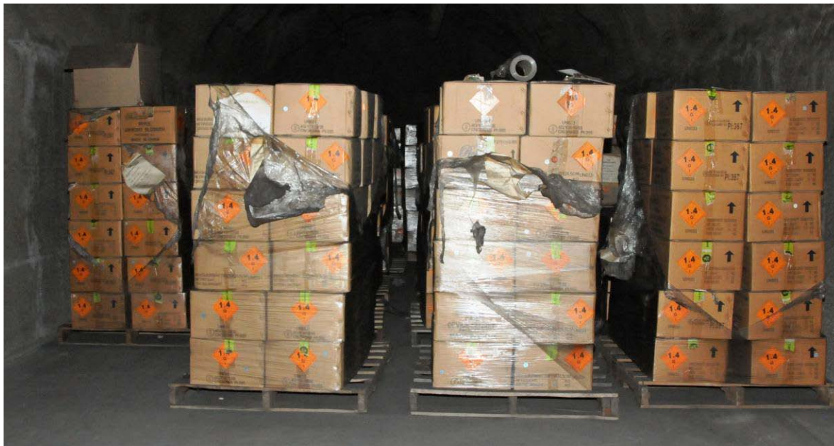
Figure 18. 2009 Seizure (second seizure) at rear of magazine, relatively undamaged with some melting of the plastic wrapping following the explosion and fire near the front of the magazine.
