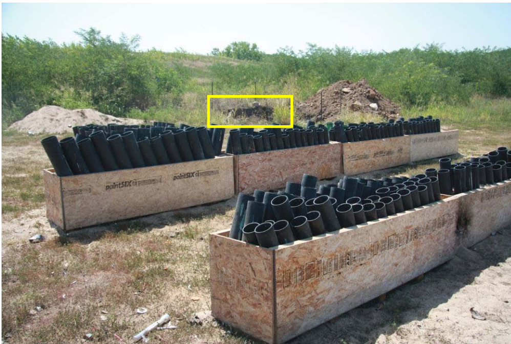
Figure 24. Sand troughs built to stabilize mortar tubes for the display show, behind which volunteers took cover during disposal activities as aerial shells were thrown into the burn pit (yellow rectangle) (courtesy of the Office of the Kansas State Fire Marshal)
