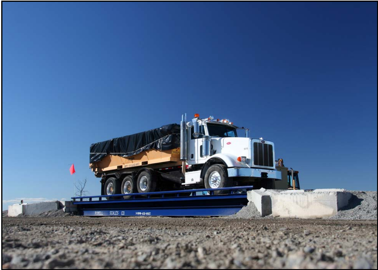
Construction and calibration of a subcontractor truck scale at 100-F Area was completed. The scale is now operational. (Photo 7)
