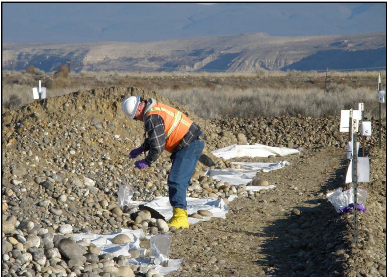
A Washington Closure Hanford subcontractor takes samples at 100-F-57, where stained concrete and soil containing hexavalent chromium was found. (Photo 10)
