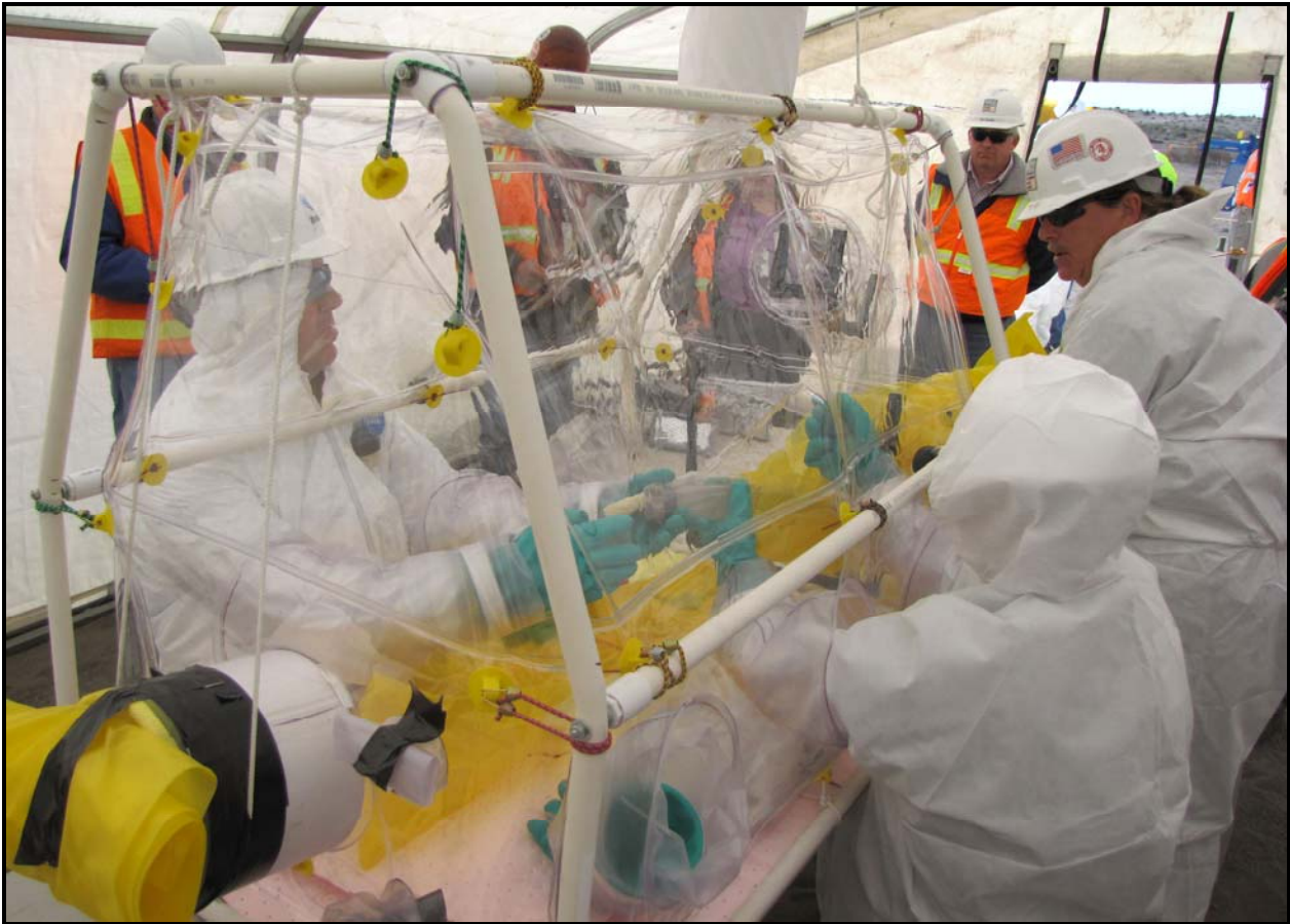
A soil sampling mockup was conducted at the 618-10 Burial Ground. Workers use a glove bag to transfer the samples to a bottle.
