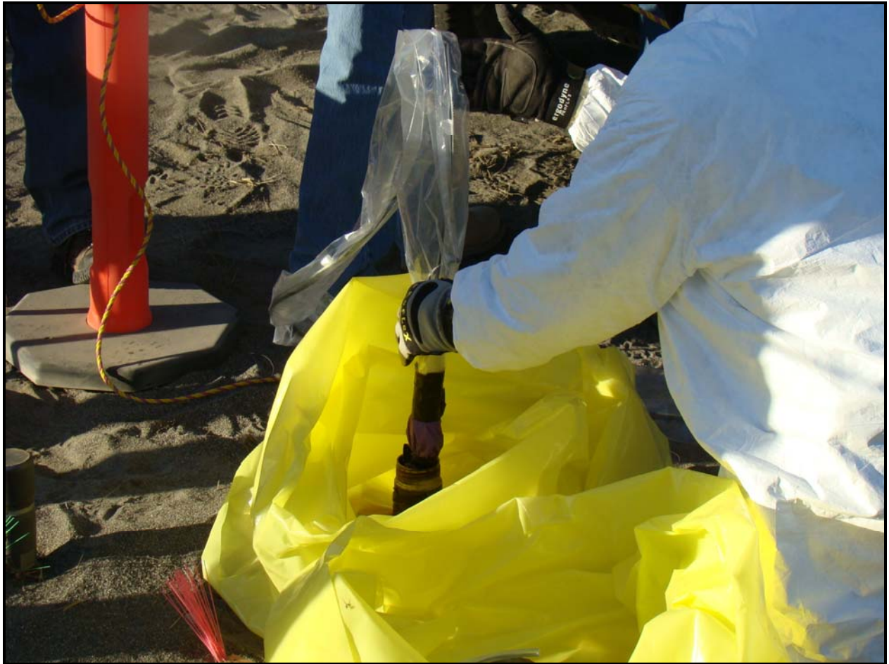
A borescope was used to inspect the affected cone penetrometer at the 618-10 Burial Ground.
