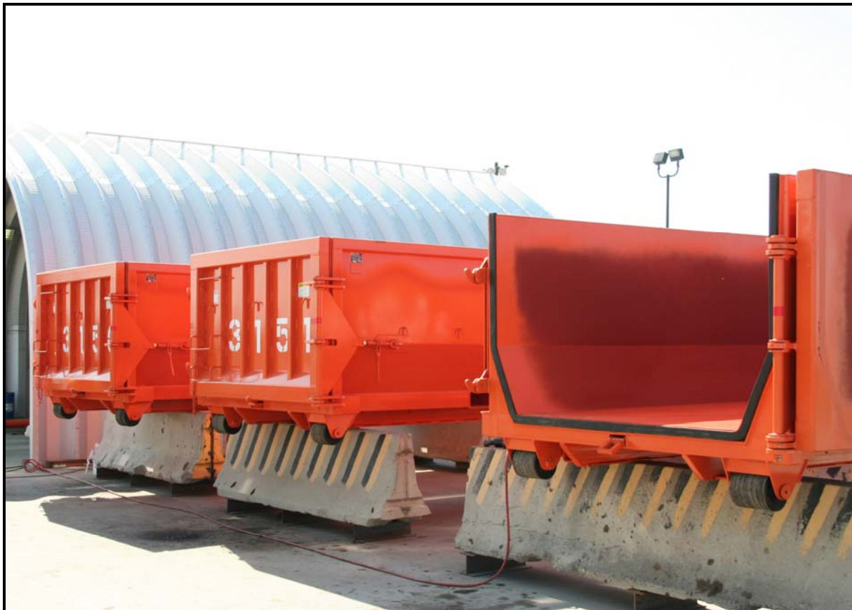
New waste containers are inspected before being placed into service. These new containers hold up to 25 tons of low-level contaminated waste.
