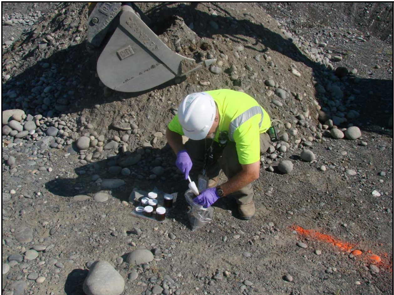
Confirmatory sampling is performed at site 100-D-88.
