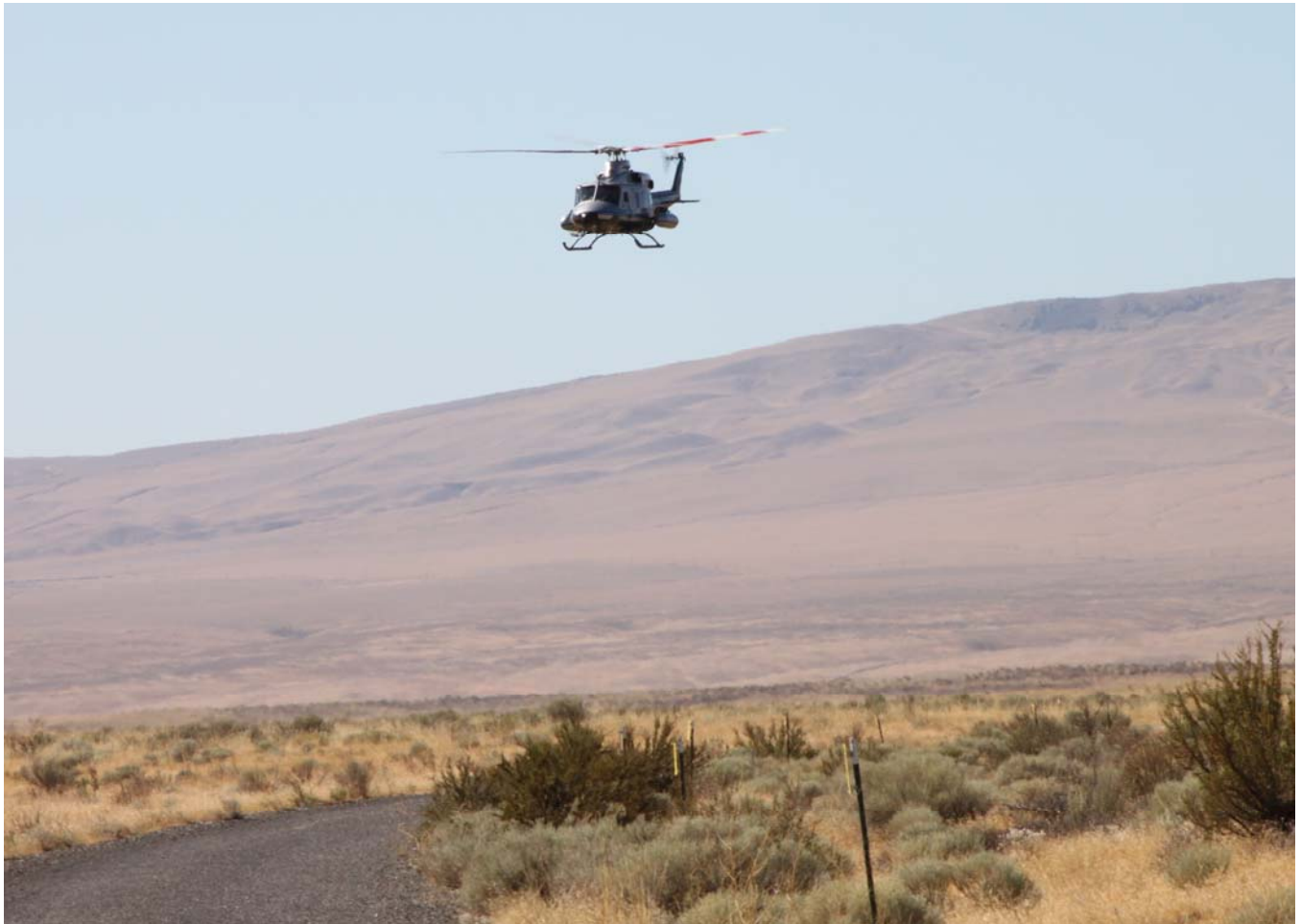
The survey was conducted at 80 miles per hour, 50 feet above ground level, to evaluate shallow soil contamination.
