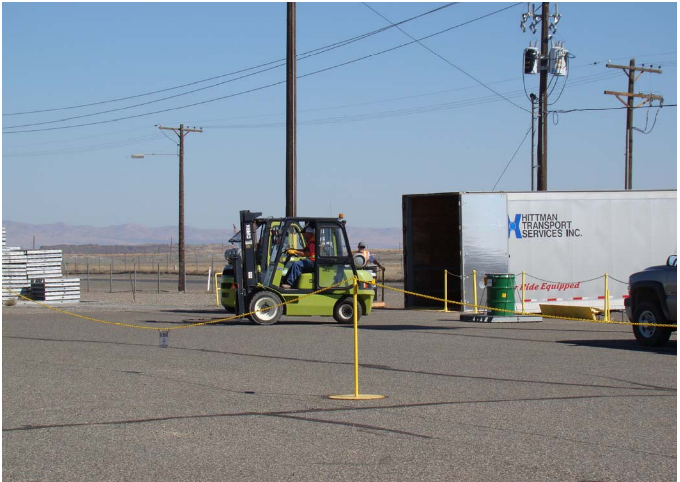
An operator at the Central Waste Complex prepares to transport drums of mixed low-level waste that were placed in overpack drums to meet Department of Transportation regulations.
