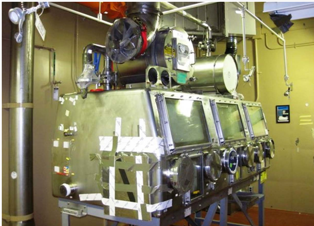
Glove box 636 in the 2736-Z/ZB Vault Complex at the Plutonium Finishing Plant before (photo 1) and after isolation of the glove box and removal of the load-in and load-out hoods (photo 2).
