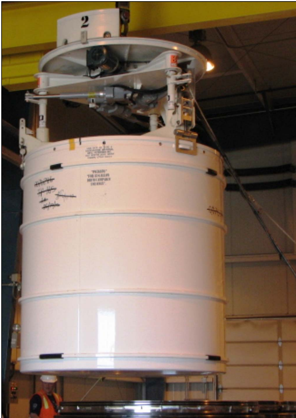
A ten-drum over-pack (TDOP), typically used for shipping ten 55-gallon drums, is modified and prepared to be loaded with four 85-gallon over-packs. Three TDOPs make up one TRUPACT-II shipment.
