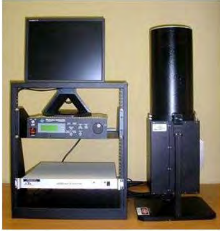
Figure 5. The micropulse lidar (MPL; left) and the Vaisala ceilometer (VCEIL; right).
