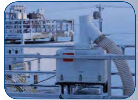
Measurements from the GVR (foreground) and the MP183A (background left) allow scientists to determine the amount of water vapor in the column of air above the site during the campaign.
