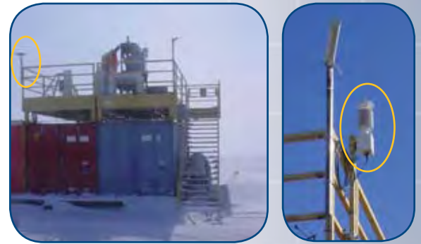
On the skydeck at Atqasuk, the new met pack (circled at right) and GPS receiver (circled at left) acquire data for the SuomiNet.
