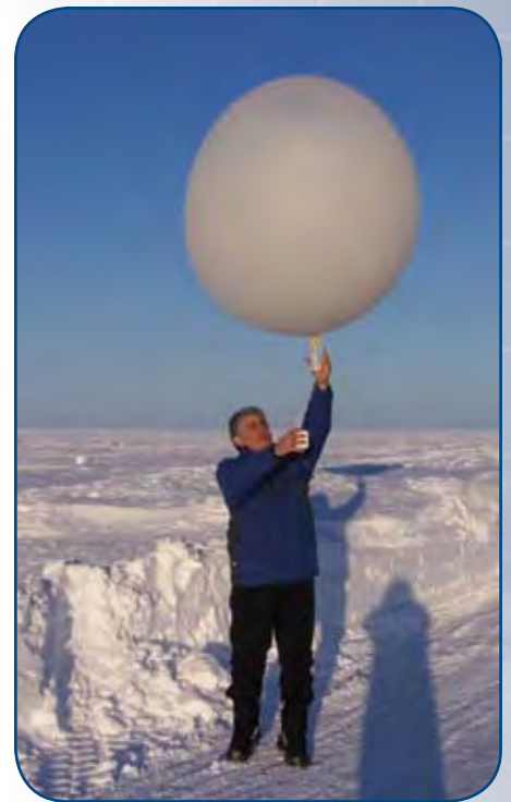
Dr. Eli Mlawer, co-leader of the field campaign, launches a radiosonde from the ACRF site in Barrow. Extra sonde launches during the 3-week experiment doubled the number of clear, dry cases in the ARM Archive, significantly increasing the statistics available for analysis.
