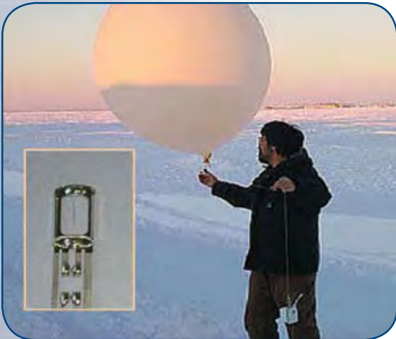
Attached to weather balloons by a string, the radiosonde package contains a variety of sensors for obtaining atmospheric data. The temperature sensor (inset) is situated at a 45-degree angle in this photo.
