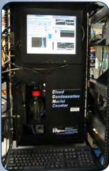
The CCN Counter consists of a vertical column with wetted walls, which provides the water vapor necessary to produce supersaturations. Particles activate into droplets when exposed to the supersaturated conditions, and the droplets are then counted by an optical particle counter.
