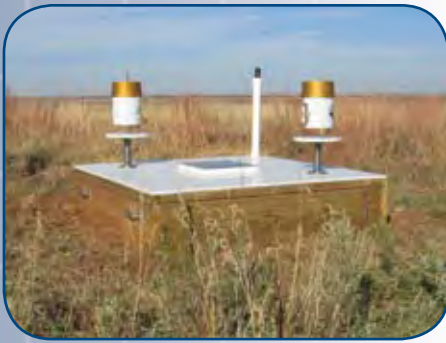
Sets of rain and stream gauges like this one are providing information about water level and flow rates from sites throughout the Whitewater River watershed during the HydroKansas field campaign.
