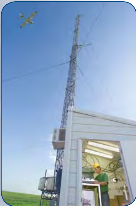
As part of the Aircraft Carbon field campaign, a set of carbon-cycle instruments and sample collection systems were added to the aircraft that routinely collect aerosol measurements at the ACRF SGP site. The airplane at upper left was collecting flasks at the same time as they were being collected at the 60-meter tower.
