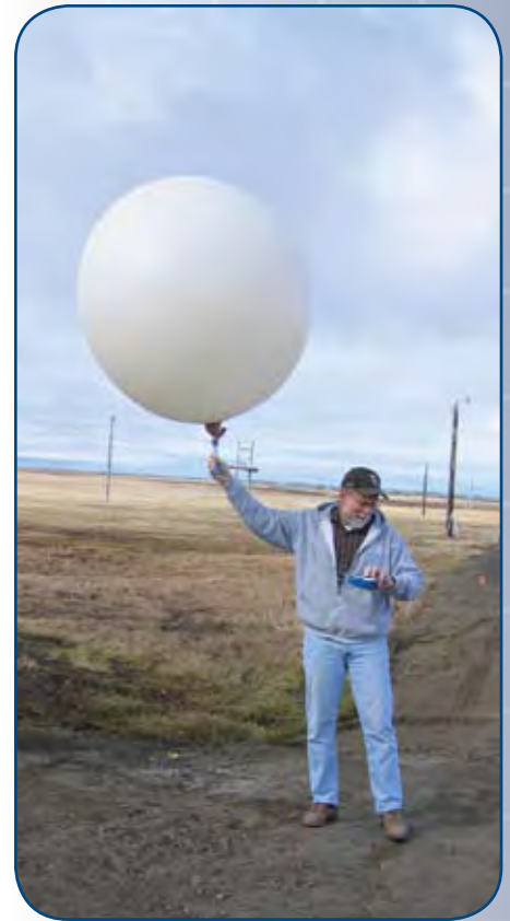
The balloon-borne sounding system consists of a small sensor package—called a radiosonde—attached by a long string to a large balloon. As the balloon rises, atmospheric measurements recorded by the radiosonde are picked up via an antenna on the ground.
