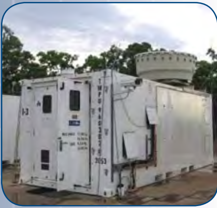
The new processor for the MMCR (antenna shown in upper right of photo) at Darwin collects spectral data in four different modes, resulting in approximately 3.4 gigabytes of signal output per day.
