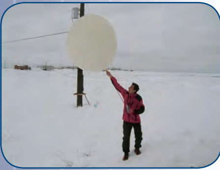
During several 5-day launch periods throughout the field campaign, M-PACE researchers released four radiosondes per day from all four experimental sites (Barrow, Oliktok Point, Atqasuk and Tulik Lake).
