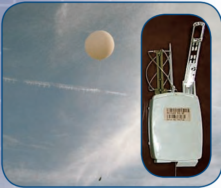
At the end of a string tied to the weather balloon, a small sensor package, called a radiosonde, contains the “brains” for measuring atmospheric temperature, pressure, and humidity.
