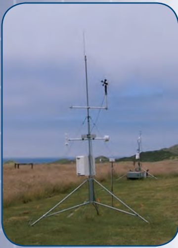
With the Pacific Ocean in the distance, a surface meteorology system collects wind, temperature, pressure, and humidity data as marine clouds drift over the field instruments at the AMF deployment site at Point Reyes National Seashore.
