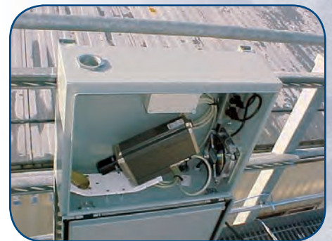
A filtered fan keeps moisture from building up on the mirror surface (bottom left) by circulating air up through the optical port (top left) of the IRT enclosure.
