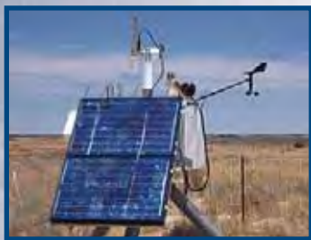
The sun photometer installed at ACRF’s Darwin site is similar to this one located in Tinga Tingana, Australia, as part of the AERONET. (Photo courtesy of NASA Goddard Space Flight Center)
