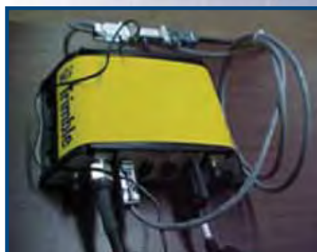
The COSMIC system, based on the Trimble netRS receiver, connects directly to a network, eliminating the need for a separate dedicated computer for communication and data transfer.
