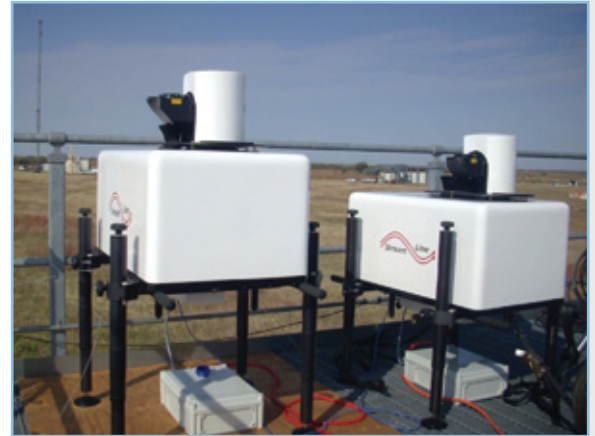
Two of the three new Doppler lidars are shown here during testing at SGP in October 2010.
