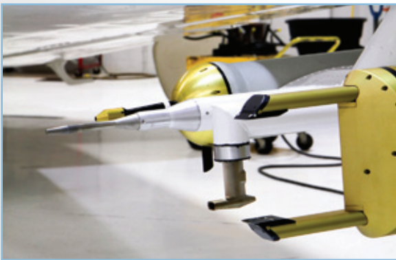
In March, ARM Aerial Facility scientist Jason Tomlinson met with colleagues at the University of North Dakota to assist in the integration of the probes onto the Citation aircraft and to provide training on the operation of the UHSAS-A (back) and HVPS-3 (front) instruments.
