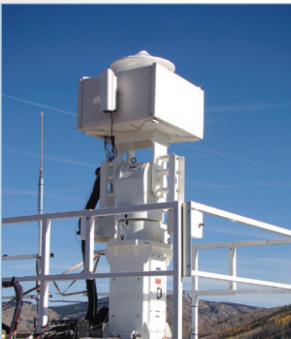
The SWACR gathered cloud properties data outside the Thunderhead Ski Lodge in Steamboat Springs, Colorado.
