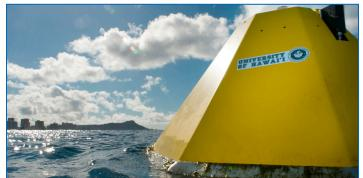
A network of offshore buoys measure variables related to ocean water quality, climate, and atmospheric conditions. This buoy off Oʻahu, Hawaiʻi is a part of the global CO<sub>2</sub> monitoring array.
