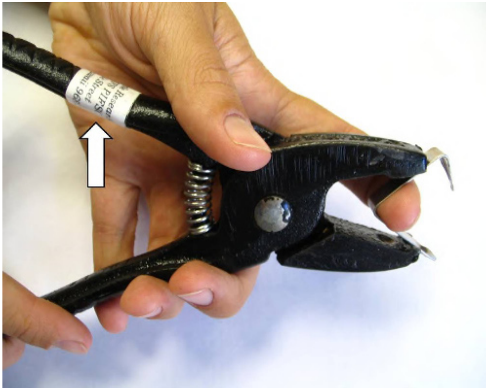
Figure 2: Loading a flipper tag into tag applicator. The arrow indicates which handle should be up.
