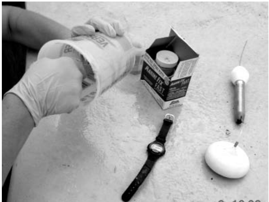
Figure 2: Mixing the epoxy compound. **Wear the latex gloves while handling the epoxy compound.**
