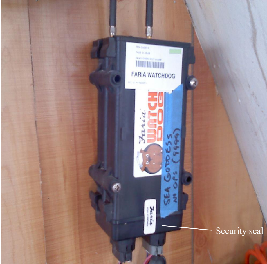
One style of VMS unit with security seal intact (sticker at bottom)
