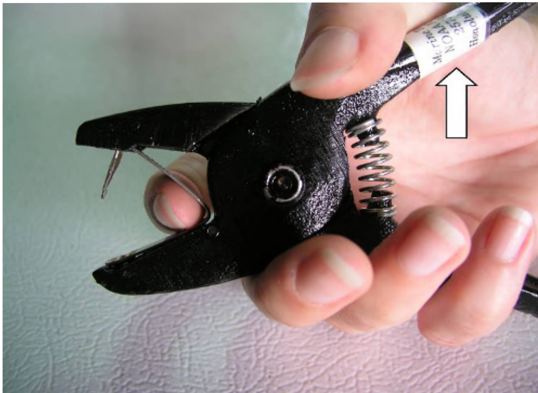
Figure 3: A fully-seated tag in the tag applicator pliers.
