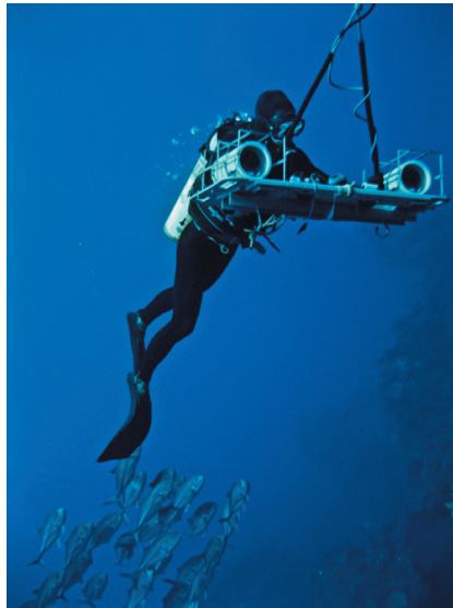
Figure 4. A modified towed-diver platform designed to capture stereoscopic images of coral reef fishes.
