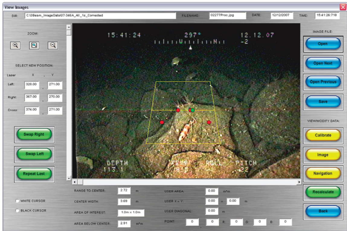
Figure 4. A screen grab from the 3Beam quantitative measurement software, enhanced to illustrate the location of the lasers on the bottom (red and green circles).
