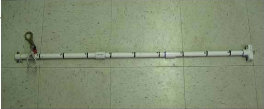
Figure 1.-- The reference tool, called a monopod, used for taking benthic photos, measuring habitat vertical relief, and estimating the outer edge of a sample cylinder.
