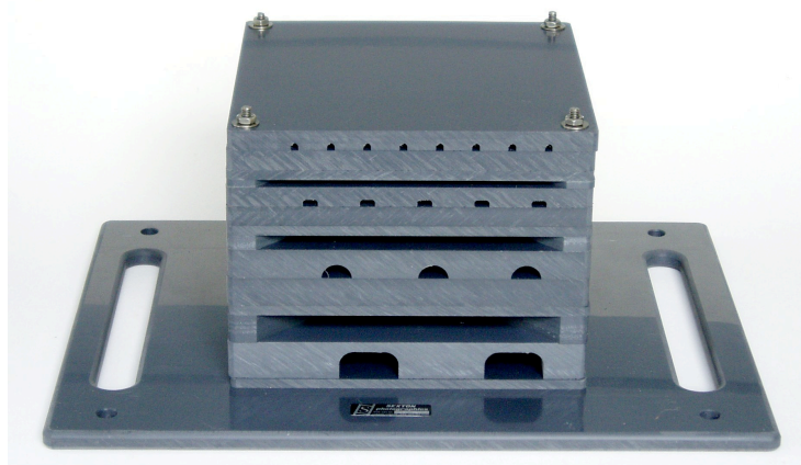
Figure 2. Picture of an Autonomous Reef Monitoring Structure (ARMS) before deployment in French Frigate Shoals.
